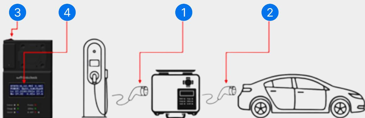
1. Displays inspection progress, CP voltage, current values, and connector pin temperatures.
